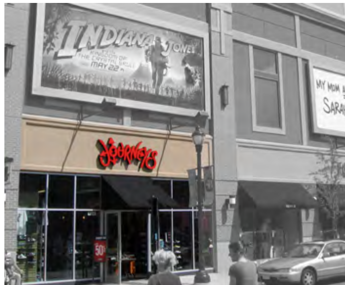
Recommended Signage Placement Signage is centered on the retail unit and between facade elements. Signage works with building design to define storefront size.
